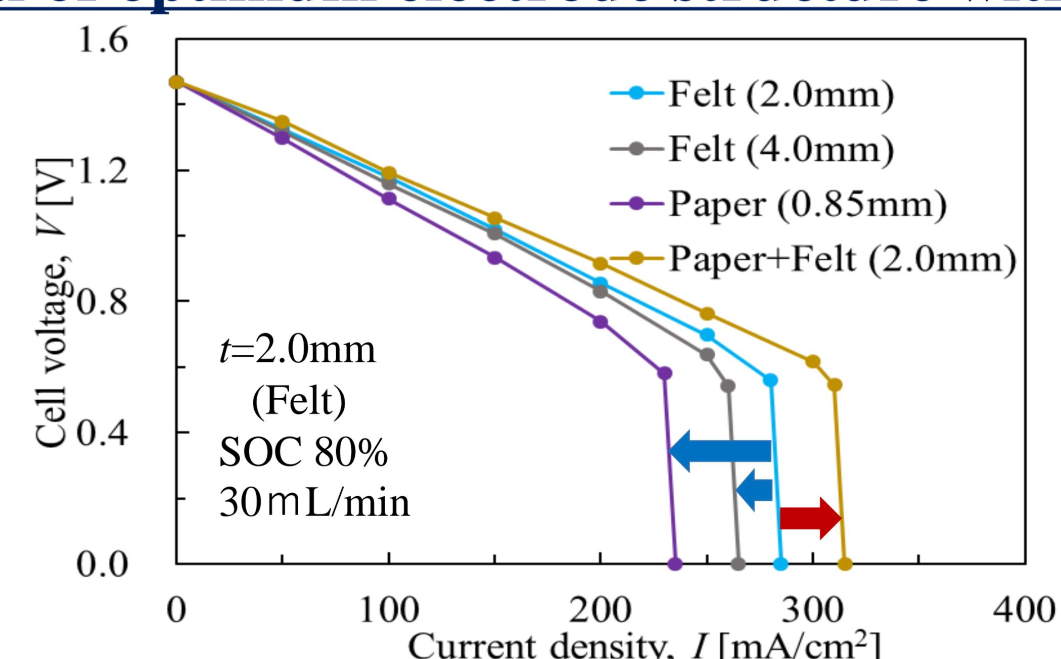
♦ Stack two felt electrodes to increase reaction surface area
