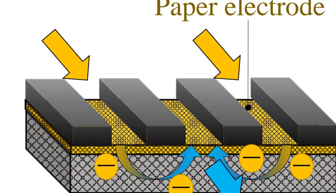
By combining the paper and felt electrode, the cell performance is improved than conventional
