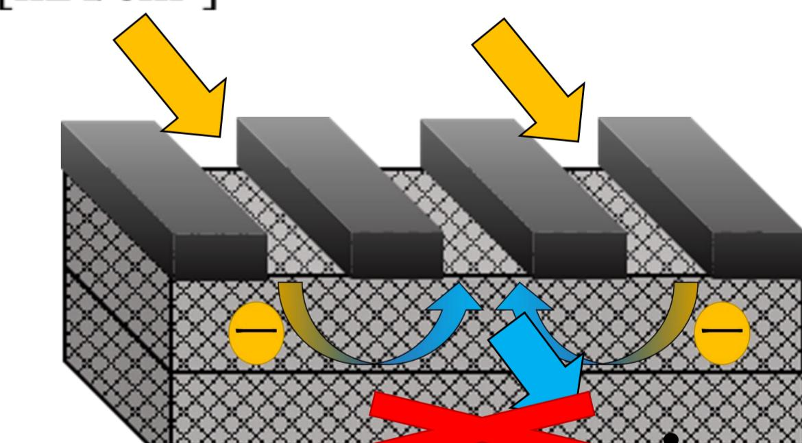
♦ Combining paper electrode with large reaction surface area on felt electrode
